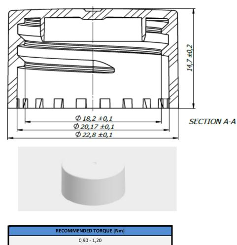
Given values of the recommended torque are approximate. The appropriate torque value for a given application depends on many factors and should be determined empirically by the customer, in conditions of the closure application.
